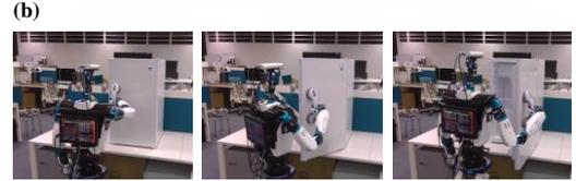
Figure 6. Results of LfO for “open a fridge.” (a) A substantiated task model with representative skill parameters. (b) Robot execution.
