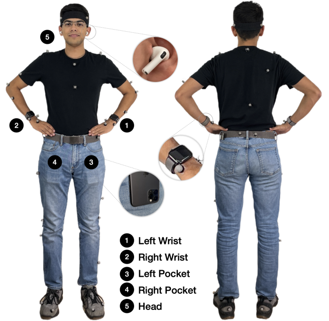
Figure 5: IMUPoser data collection setup. Participants wore 2 smartwatches, kept 2 smartphones in their front pockets, and wore wireless earbuds. 41 retroreflective motion capture markers were also placed around the body to track ground truth body pose.
